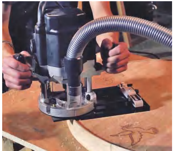
▲ Pic.18 Creating a high quality finish on the lath using Trend's multifunctional CRB combination router base
